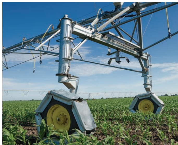
Hydraulic motors are coupled directly to the planetary wheel hub allowing a narrower travel profile for reduced crop loss.
