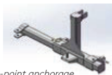
Three-point anchorage central and offset hitch
