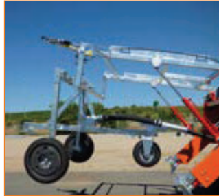
2000 series articulated trolley and hydraulic lifting frame
