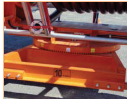
Hydraulic rotation of the turntable
