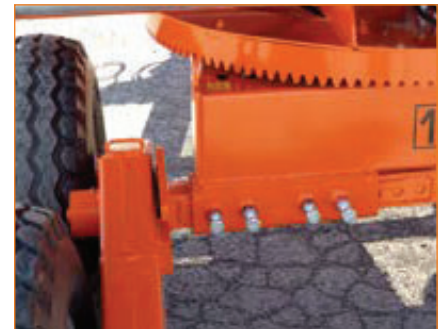
Adjustable tandem axle
