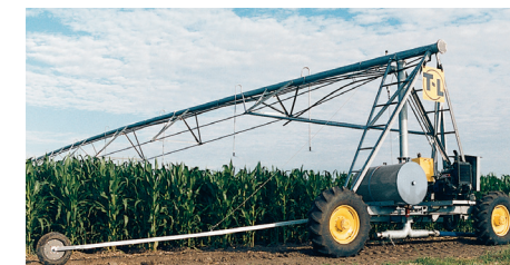
One Span Linear system (with hose drag and furrow guidance)
