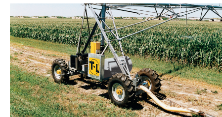
Center-feed or end-feed hose drag linear (with buried wire or above ground cable guidance)
