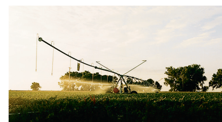
One Span Linear (with furrow guidance)
